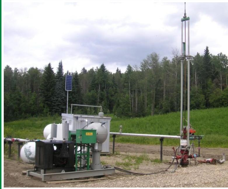
*Ecoquip Pump Jack installed and operating on-site*
